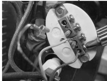
Slide wires out through the white plastic ties on the hinge.
