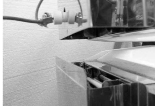
Remove the lid and put it aside. Then unlatch each of the clips around the body.
